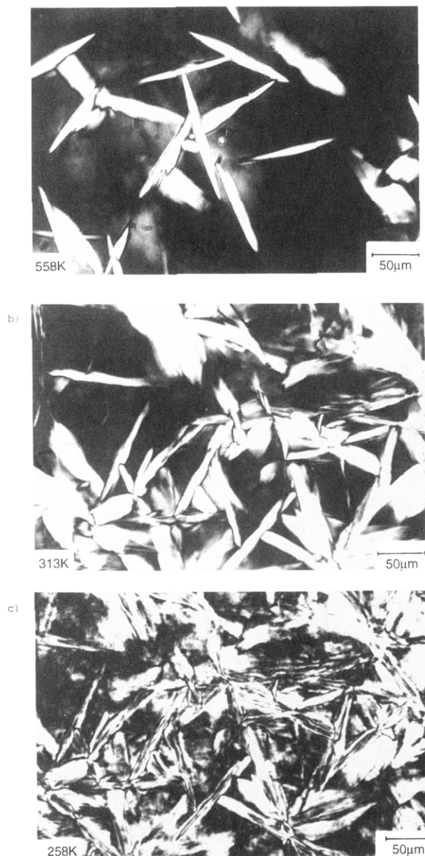
Figure 5. Optical polarizing micrographs of poly(di- n -hexylsiloxane) upon cooling from the melt: (a) below the isotropization transition; (b) above the upper disordering transition; (c) in between the upper and the lower disordering transition.
