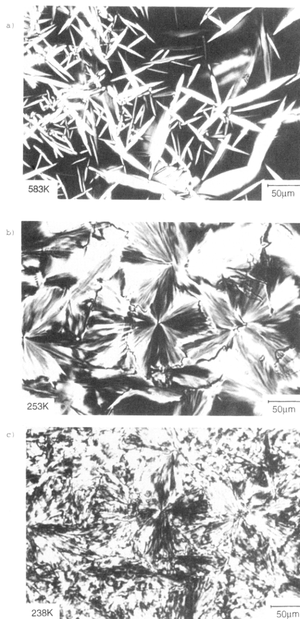
Figure 4. Optical polarizing micrographs of poly(di- n -pentylsiloxane) upon cooling from the melt: (a) below the isotropization transition; (b) above the upper disordering transition; (c) in between the upper and the lower disordering transition.
